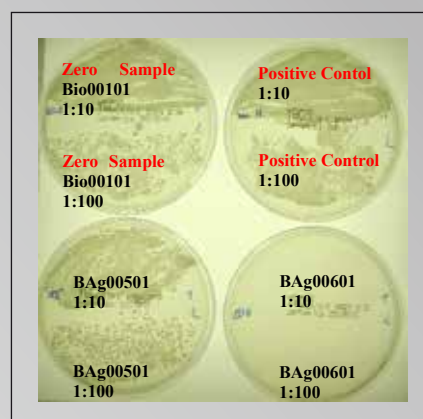
Figure 7: Result of incubated diluted crop-out of the samples. No fungal attack on treated samples BAg00601.
